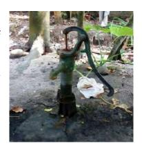
district, a type of filter pipe, locally known as champ pipe, just 3 to 4 meters deep from the ground fitted with either motor or hand pump.
